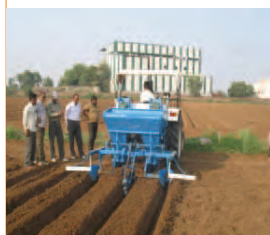
Field testing of potato planter
